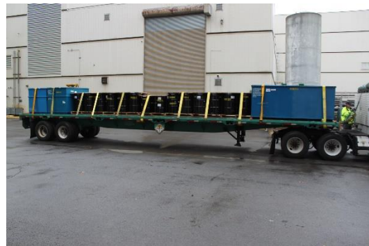
Exhibit 5-6. Truck with B-boxes and drums for shipping LLW to Energy Solutions
