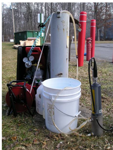
Exhibit 6-5. Well Monitoring Set-up
