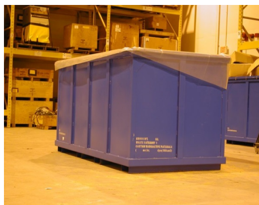
Exhibit 5-6. B-box with Liner in RWHF for Shipping Radioactive Waste for disposal.
