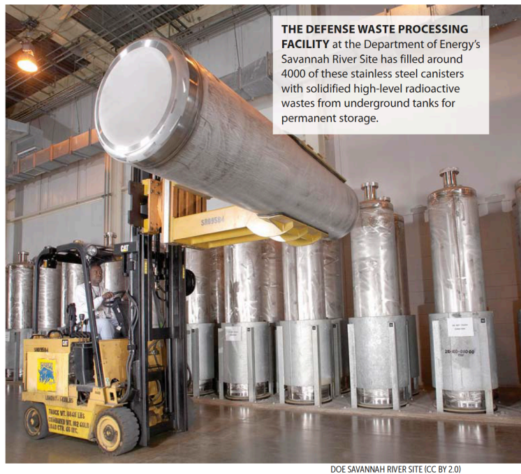
Fig. 4.4 – handling of high-level waste canisters (from [2])
