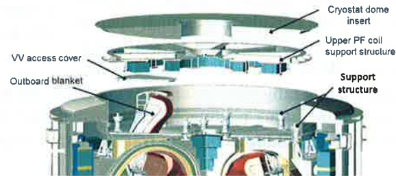
Figure 2b. Local details of upper cryostat
