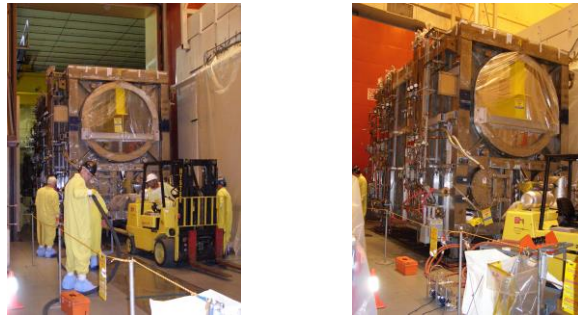
Fig. 2. The 40 Ton Neutral Beam Box being Transported using Air Casters
