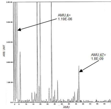
Fig. 4. RGA reading of the vessel exhaust during boronization
