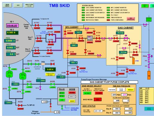
Fig. 3 The PLC page of the fully automated dTMB boronization process for NSTX-U
