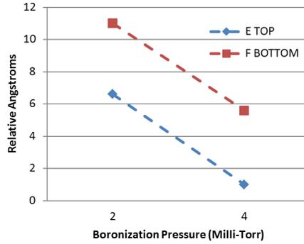
Fig 4. Coating thickness at Bay F bottom and Bay E top under boronization pressure of 2 and 4 millitorr
