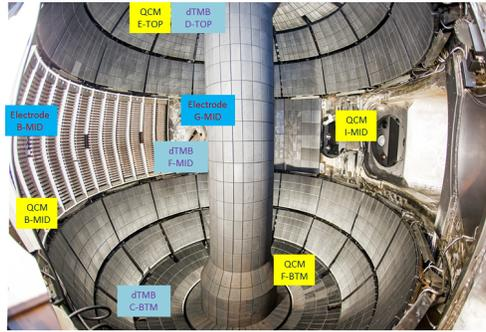
Fig. 2. Physical location of the dTMB injection ports, the glow discharge electrodes and the QCMs on the inner wall of NSTX-U vessel. Picture is taken from the Bay A neutral beam port.
