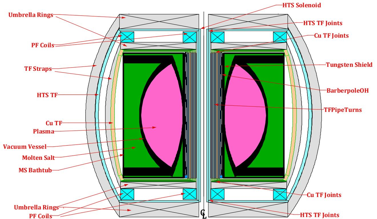
Fig. 8. DT Fusion Neutron Source for HMSR
