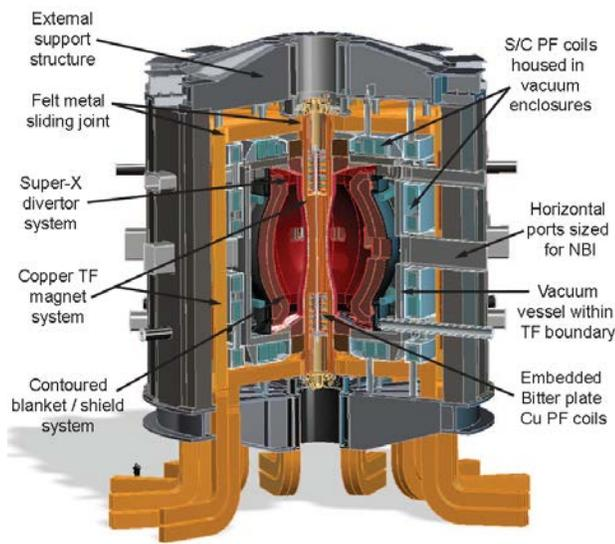
Fig. 3. FNSF with 1-turn Copper TF, No Solenoid
