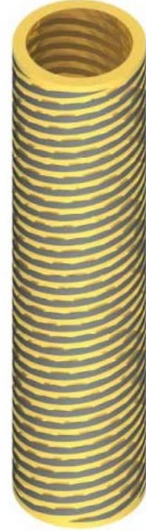
Fig. 6. Barberpole All-Metal Solenoid
