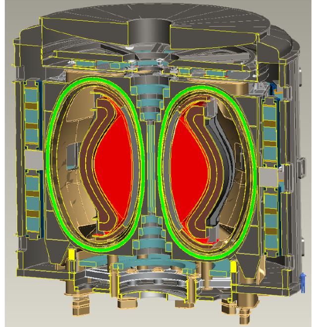
Fig. 4. FNSF with HTS TF and Small Solenoid
