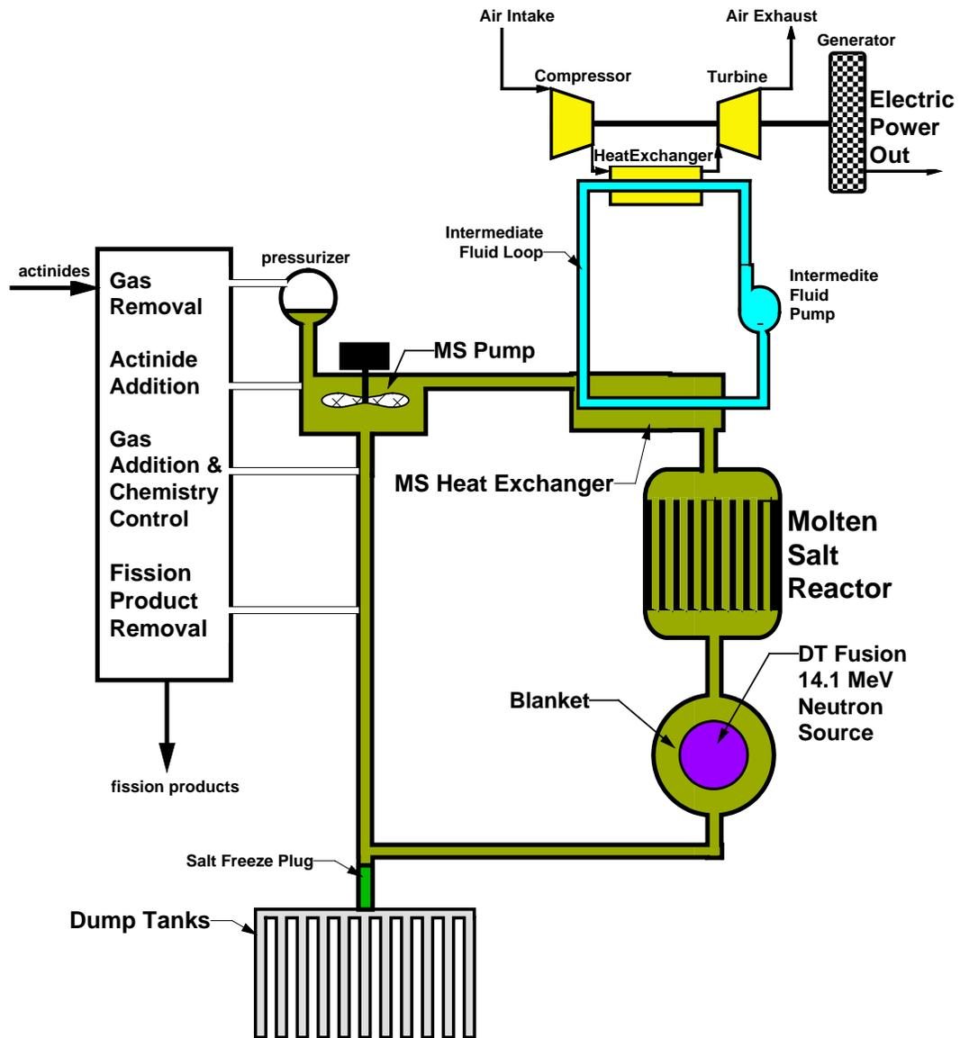
Fig. 1. Hybrid Molten Salt Reactor (HMSR) Configuration
