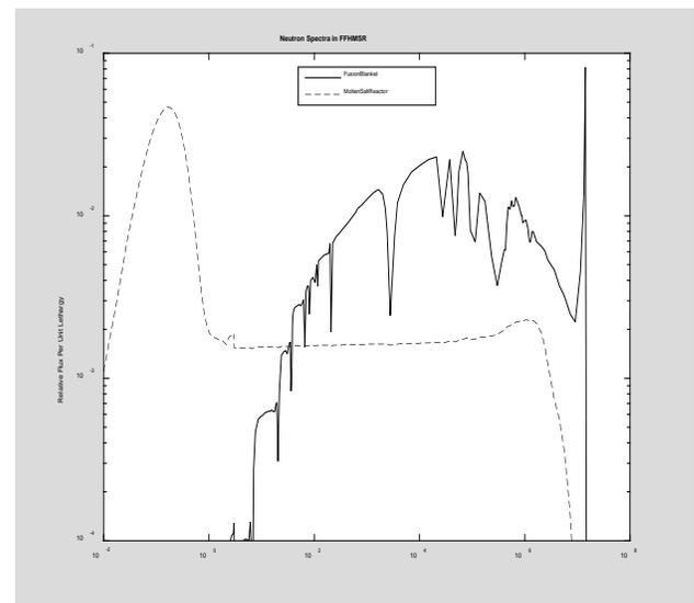
Fig. 2. Lethargy Plot of Neutron Spectra in HMSR
