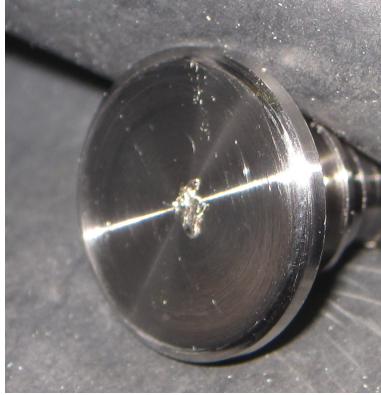
Fig. 2 Photograph of a particle of lithium pressed onto a 13 mm diameter stainless steel SAM stub.
