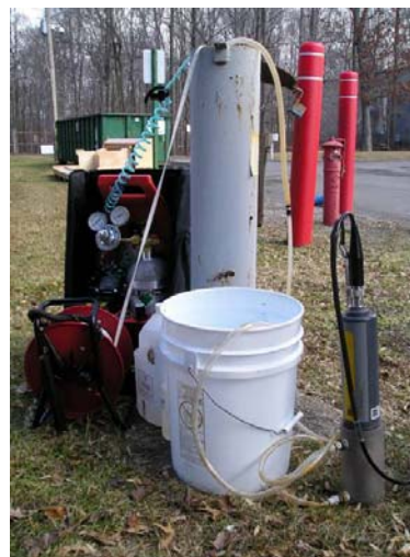
Exhibit 6-5. Well Monitoring Setup (Compressed Air, Water Depth. Meter, Discharge Collection Bucket, Probe)
