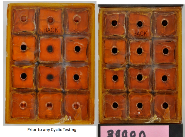
Fig. 16 CTD Tensile Strain Controlled Test, Aligned Sample
