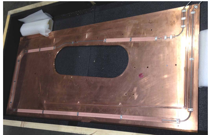
Fig. 14. As-delivered copper plate with plasma sprayed 316SS cooling tubes and thermocouple grooves
