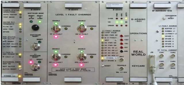
Fig. 17. DCPS Interconnection Subsystem Hardware User Interface
