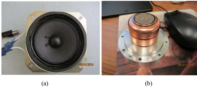
Fig. 12. (a) 8- \Omega 15 W speaker driven with a square pulse into an audio amplifier to mimic the arcing sound; (b) CMI-5247TF-K Microphone of CUI Inc. in a copper enclosure to reduce the EMI during an arc.
