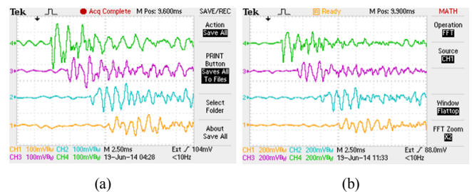
Fig. 14. The microphones signals while the blower was at 25% of the full power; (a) the transmission line was under 1 bar pressure, (b) the transmission line was under 3 bar pressure.
