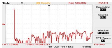
Fig. 17. The power spectrum from the microphones signals while the transmission line was under 3 bar pressure with blower off.
