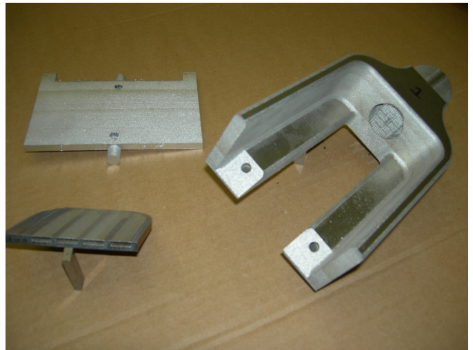
Fig. 9. Fork and mirror are printed to near-final dimensions
