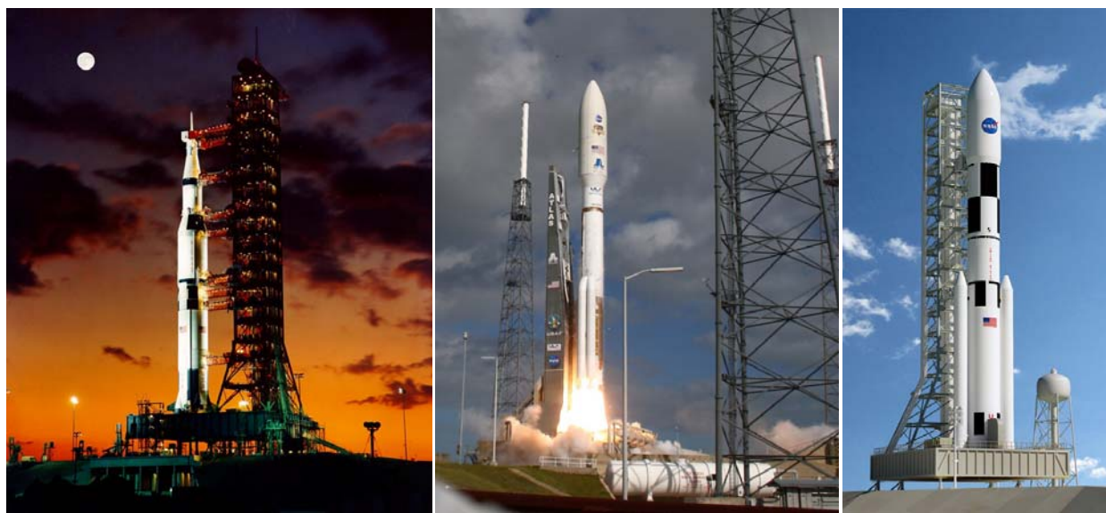
Figure 3. (Credit NASA). Examples of the best heavy lift chemical rockets: Apollo 11 Saturn V vehicle sitting on the pad (left), with third stage J2 engine specific impulse of 420 seconds, and thrust of 1,000 kN. The Mars Curiosity rover at launch on an Atlas V rocket (middle). NASA's new Space Launch Systems heavy launch vehicle (right).
