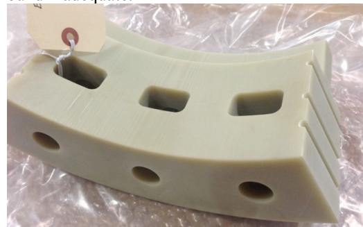
Figure 11 Crown Segment Machined from High Pressure Laminate
