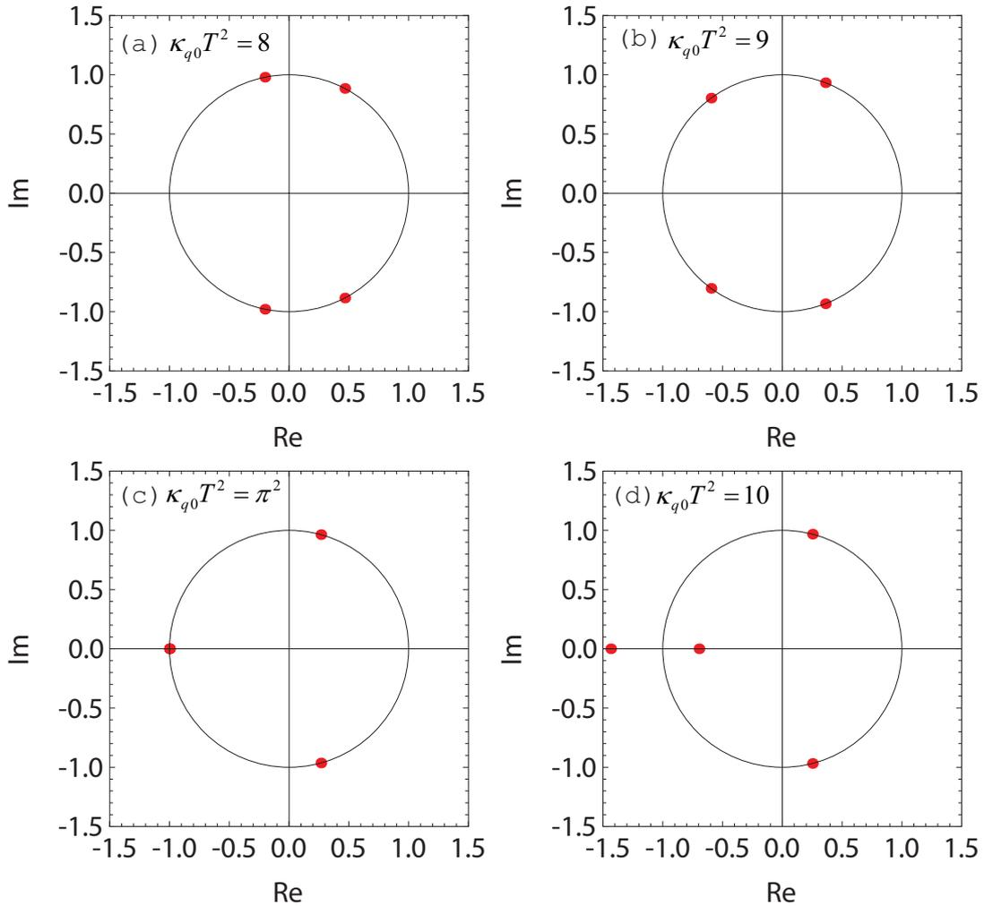
Figure 3: Eigenvalues of continuously rotating quadrupole lattices. The two eigenvalues on the left half circle have different signatures in (a), and move towards one other as  $\kappa_{q_0} T^2$  increases in (b). The Krein collision occurs at  $\kappa_{q_0} T^2 = \pi^2$  in (c), after which these two eigenvalues on the left move off the unit circle and lead to an unstable lattice in (d).
