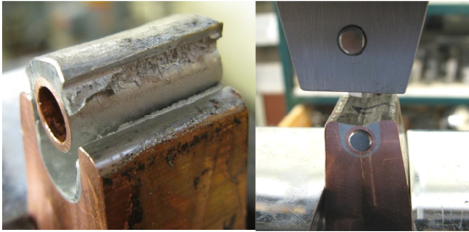
Figure 6 Tensile Strength Testing of Production Solder Paste
