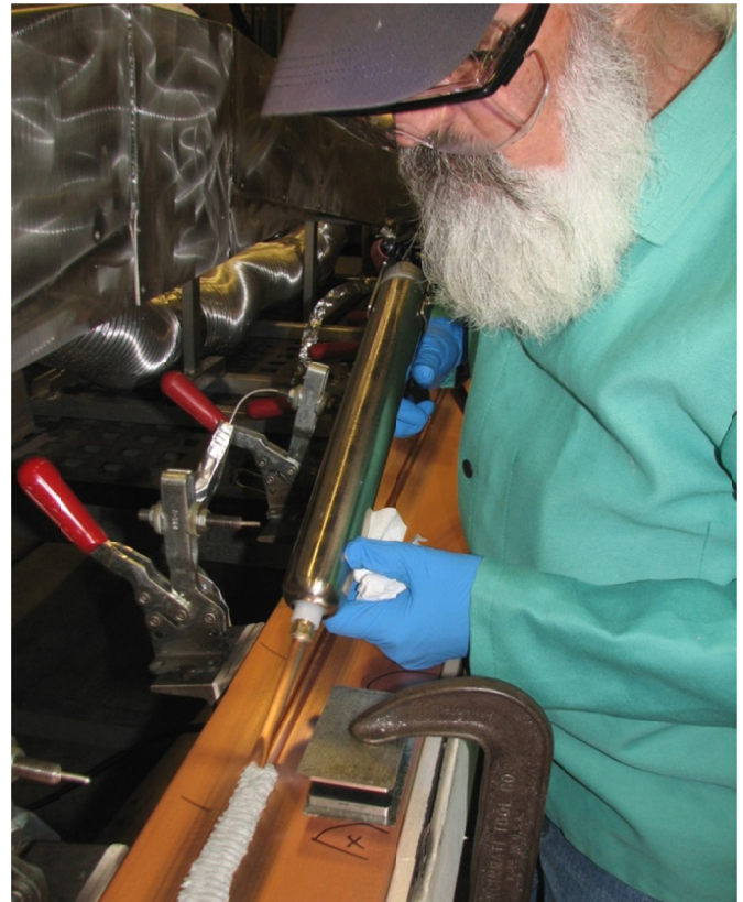
Figure 27 Apply Solder Paste with Pneumatic Applicator
