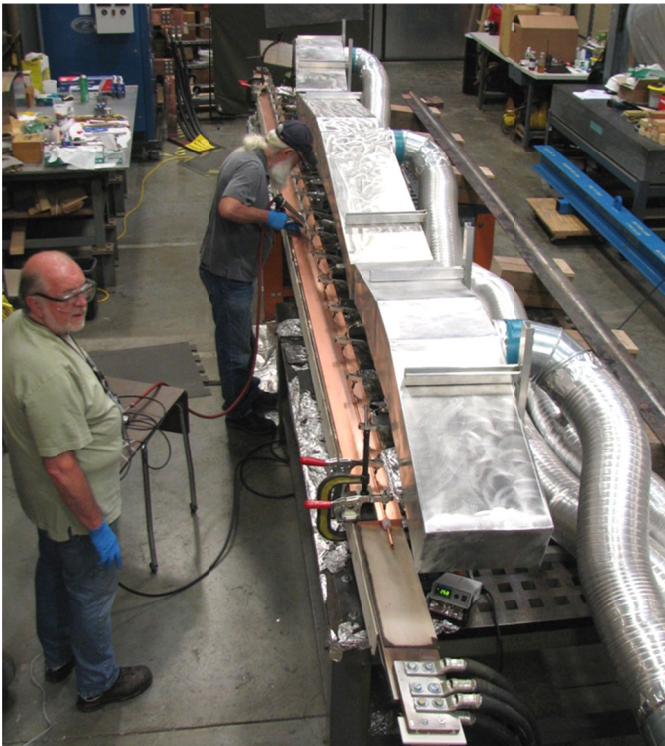
Figure 19 Production Station with Fume Exhaust Hoods
