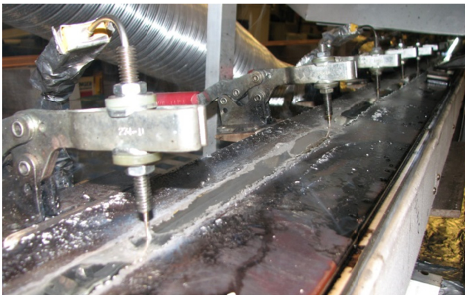
Figure 29 Solder Skimmed & Tubes Agitated
