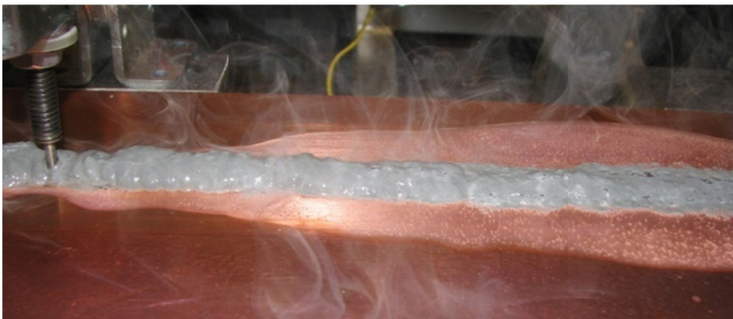
Figure 28. Flux Liquifying as Paste is Heated
