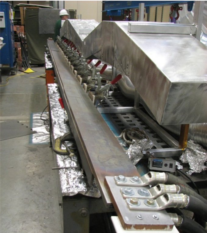
Figure 16 Completed Production Soldering Station
