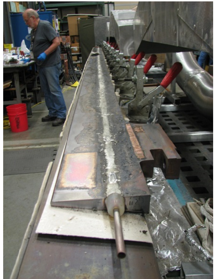
Figure 30 TF Conductor Ready for Grinding Operation
