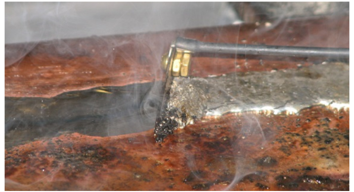
Figure 8 Scale Skimming of Molten Solder
