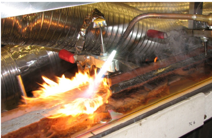
Figure 7 Reducing Flame Disassociating Copper, Tin & Silver Oxides
