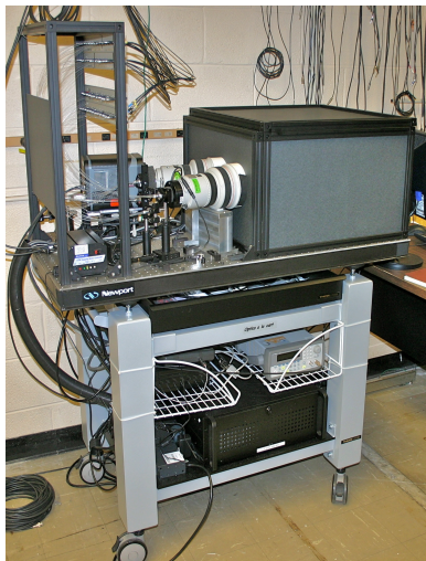
FIG. 2. Spectrometer, computer, and all associated hardware are shown on mobile cart at LTX facility.
