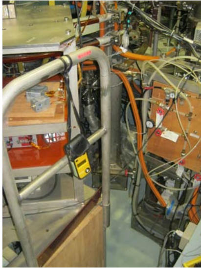
Figure 4a. An oxygen monitor hanging at the entryway to the TST-2 tokamak pit.
