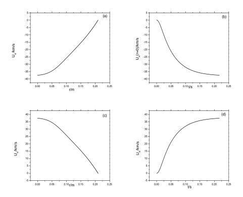
FIG. 2: (a) Radial profile of rotation speed with  $q_e n_{er} u_{er}^r = -0.25 A/m^2$ . (b) Time history of the rotation speed at plasma core for the same case as (a). (c) Radial profile of rotation speed with  $q_e n_{er} u_{er}^r = 0.25 A/m^2$ . (d) Time history of the rotation speed at plasma core for the same case as (c).
