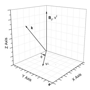
FIG. 1: Plasma exists in the region of 0 < y < a. A constant and uniform magnetic field is in z direction, and lower hybrid waves propagate within the x - z plane.
