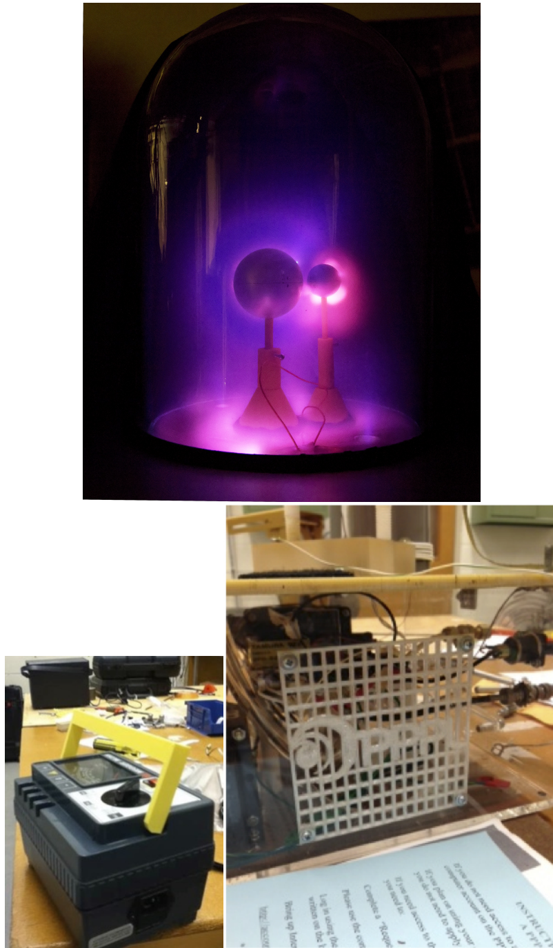
FIG. 4. Photographs of printed parts in a) Planeterrella holding up aluminum spheres, b) replacement handle, and c) protective cover.
