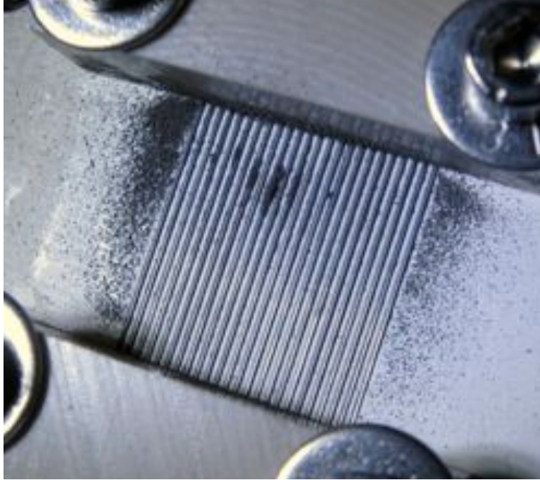
Fig. 12: Rectangular detector after dust deposition while energized to 200V.
