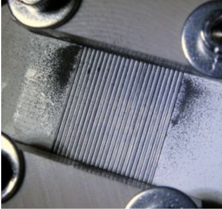
Fig. 13. Rectangular detector after dust deposition while energized to 250V.
