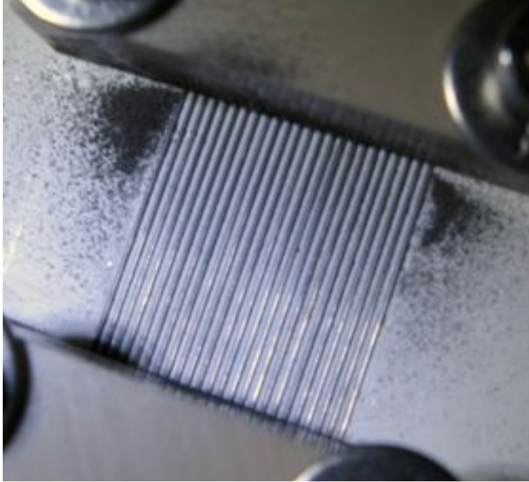
Fig. 14: Rectangular detector after deposition while energized to 300V.
