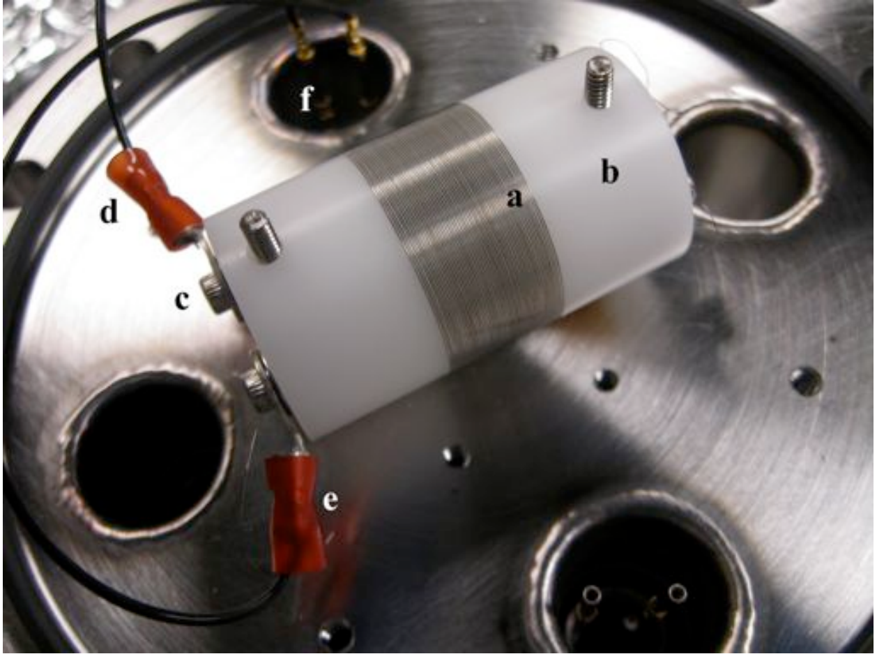
Fig. 5: Cylindrical detector assembly on flange: (a) two 0.13mm tungsten wires arranged in a double helix, (b) Delrin cylinder, (c) screw securing tungsten wire to external connector, (d) wire connecting to power supply, (e) wire connecting to detection circuitry, (f) feed-through.
