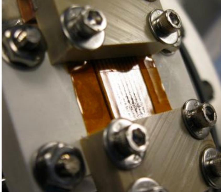
Fig. 16: Dust deposition on a rectangular detector whose wires were covered with insulating tape. Dust has lined up along the wires that were at high voltage. (Note: this particular detector had wire diameters and spacing of 0.50 mm, twice that of the rectangular detector referred to by default in this paper.)
