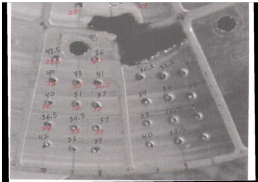
Fig. 5. Rockwell tests were performed on conductors to rule out fatigue
