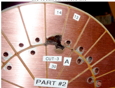
Fig. 2. Coil slice showing the origin of short
