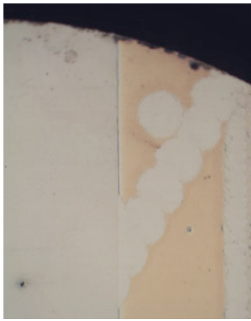
Fig. 5 Individual laser pulses at 1.8 \text{ J/cm}^2 are effective at cleaning a 166 nm carbon coating as shown in the diagonal track. The broad band on the left is the uncoated reference.
