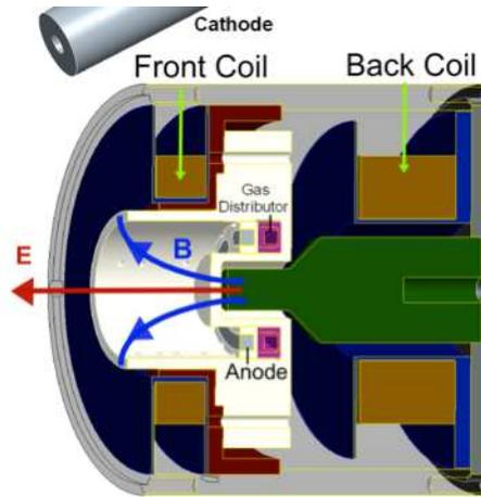
Figure 1. Schematic of a cylindrical Hall thruster.
