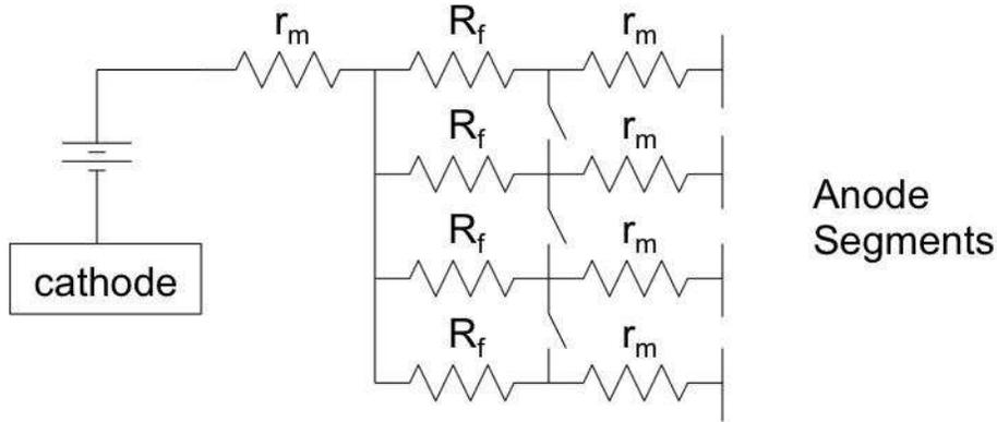
Figure 2. The feedback was implemented by attaching resistors between each anode segment and the thruster power supply. The feedback resistors,  $R_f$ , were either  $100\Omega$ ,  $200\Omega$ , or  $300\Omega$  and the measurement resistors,  $r_m$ , were  $1\Omega$ .
