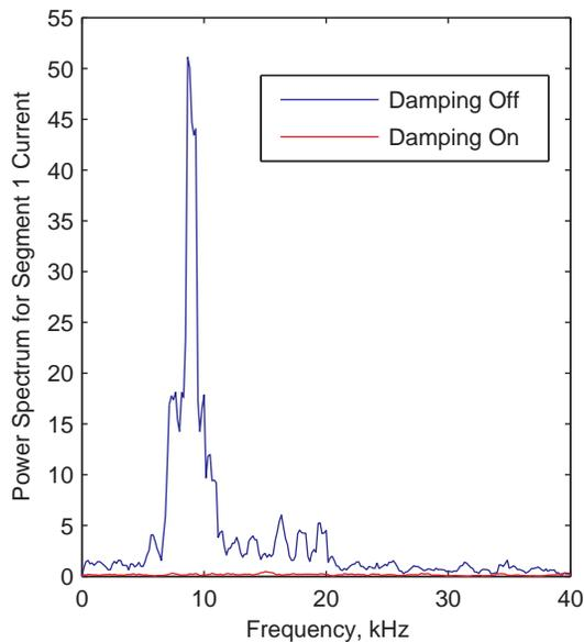
Figure 4. Fourier transform of the current to Segment 1 of the thruster when the damping is off compared to when it is on.
