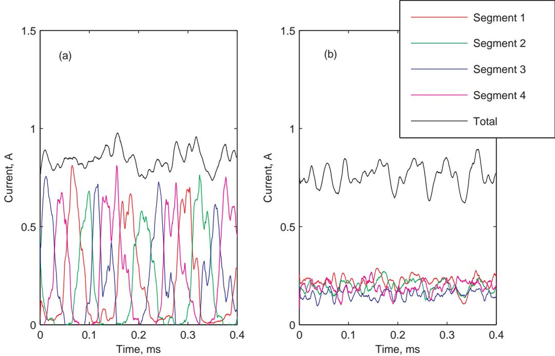
Figure 3. Total discharge current and current through each anode segment for the case when the damping is off (a) and the case when it is on (b). The damping strongly suppresses the oscillations which can be seen in the segment currents when the damping is off.
