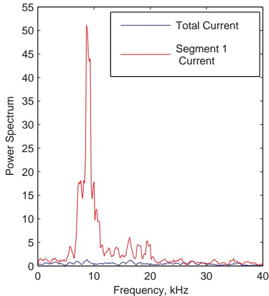
Figure 5. Fourier transform of the total current compared to the transform of the current through an individual segment. The large coherent oscillation at around 10 kHz in the segment current is absent in the total current.
