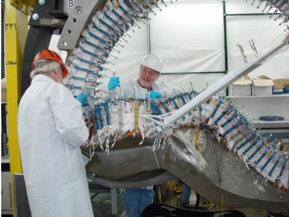
Figure 5: Modular coil winding operations at PPPL.
