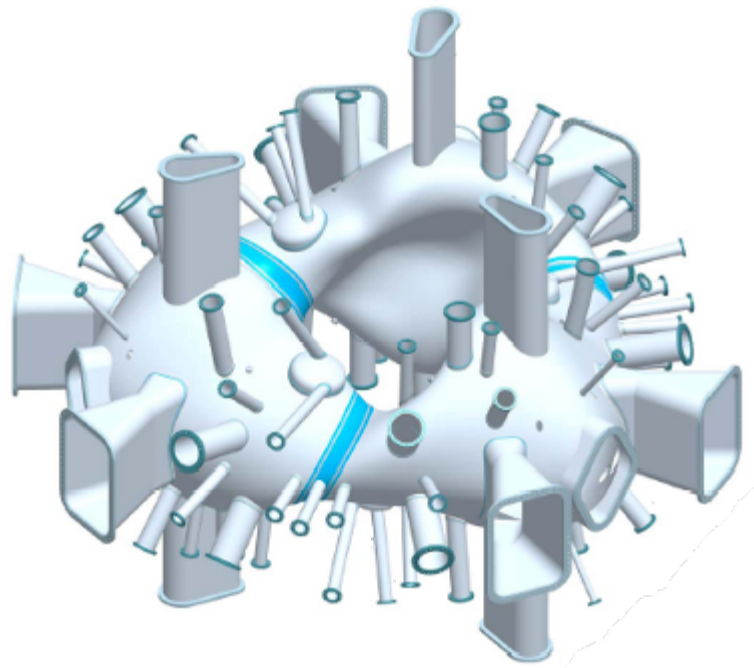
Figure 2: NCSX vacuum vessel design
