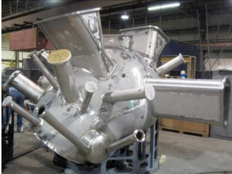
Figure 3: One of three NCSX vacuum vessel sectors fabricated by industry and delivered to PPPL. (The port extensions were later temporarily removed during assembly operations.)
