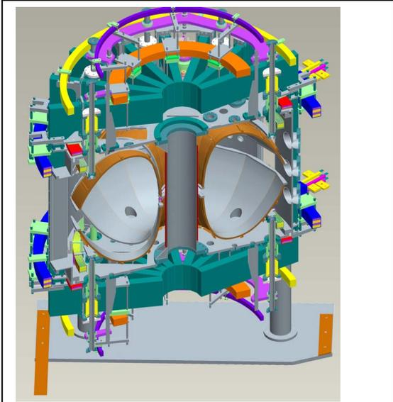
Figure 3. Section of the LTX machine showing the installed shell sections
