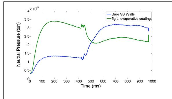
Figure 8. Comparison of machine pressure with and without lithium
