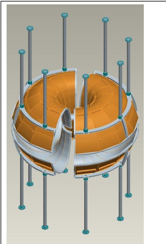
Figure 4. Shows the configuration of the four shells independent of the other machine elements
