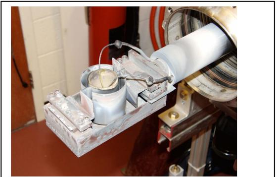
Figure 6. Used evaporator prior to cleaning
