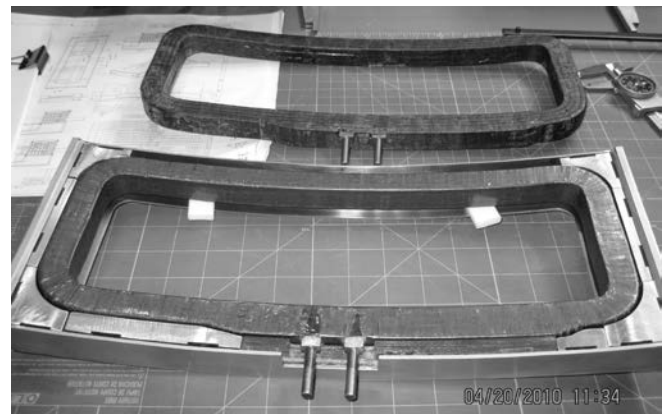
Figure 8 Cured coil wrapped in Kapton positioned into the case top
