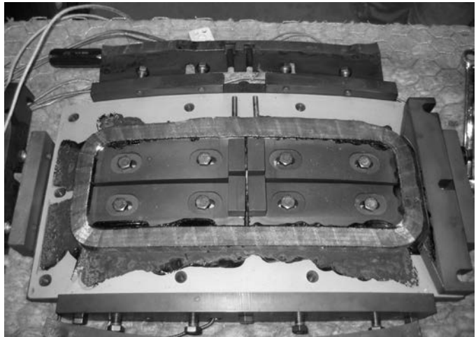
Figure 5 Mold opened revealing cured coil, four inside mold pusher blocks, copper sheet, and excess resin
