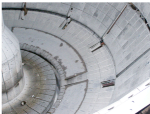
Fig.12. View of lower divertor region showing LLD and surrounding graphite tiles. The dark regions at the edges of the LLD plates exhibit sputtered graphite deposition due to arcing.
