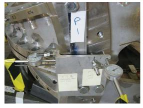
Measurements were retaken and the spreadsheet would readout the required changes in X, Y, Z directions to achieve acceptable alignment. Once the X and Y directions were aligned, the coil was then lifted or jacked when possible and surrogate shims were installed to set the correct Z position. These allowed the actual coil winding centers to be quickly realigned within the required tolerance.
