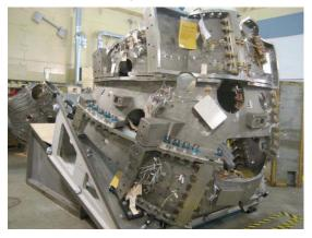
This allowed us to transfer the coils with the first wedge and not disturb the coordinate system. This worked fairly well accept that the top wedge settled a few thousands of an inch after a few days. It was determined that the shims that the leading edge of the top wedge was placed on were a bit too compliant.
