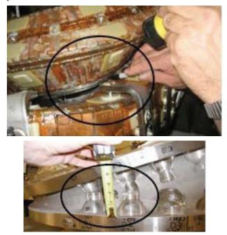
The only solution was to proceed with a 100% pre-fit of mating coils. After a few pre-fits, it was determined that this was a significant undertaking worthy of assigning a separate work crew and engineer in charge. Fortunately, the foresight to check into this issue avoided significant assembly delays. The coils were thoroughly checked and hand ground where needed until at least  $\frac{1}{4}$ " clearance was available. The coils were then delivered to the FPA crews ready for assembly.
