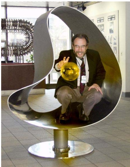
Exhibit 2-5. NCSX Vacuum Vessel Prototype (note its unique shape)
