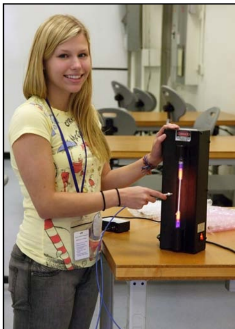
High school research intern Lauren Chilton calibrating a visible spectrometer for her project: Temperature Measurements of an Electron Cyclotron Resonant Source via Visible Spectroscopy.
