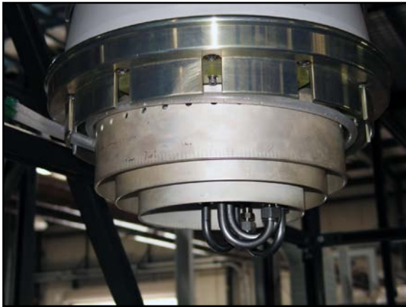
Figure 3. Socket assembly for the new high-power EIMAC tube for one of the ICRF transmitters on DIII-D capable of delivering 2 MW of fast-wave power into the plasma at approximately 100 MHz.
