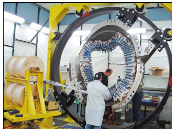
Figure 2. Winding of an NCSX modular coil on the Modular Coil Winding Form (WCWF) at the Princeton Plasma Physics Laboratory.
