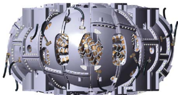
Figure 3. (Top) Completed NCSX modular coil. (Bottom) Completed toroidal structure shell.
