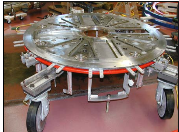
Figure 3. Lower vacuum vessel lid showing external coil mounting structures and new poloidal-field coil (red). The wheels are attached temporarily to allow ease of movement from the assembly area to the machine room where LTX will be operated.
