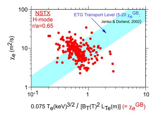
Figure 18:  $\chi_e$  as a function of  $\chi_{e,GyroBohm}$  for a collection of NSTX H-mode discharges at r/a=0.65. The blue shaded region indicates the theoretically expected range of  $chi_e$  that would be consistent with ETG-driven transport (5 to 20 times  $\chi_{e,GyroBohm}$ ).
