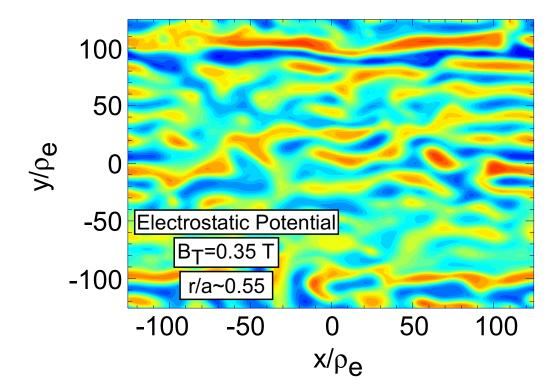
Figure 13: Results from a non-linear fluid calculation with finite Larmor radius corrections of the 0.35 T discharge at r/a=0.55. The calculation shows the formation of radial streamers with radial extents of  $200\rho_e$  ( $\sim 2$  cm).
