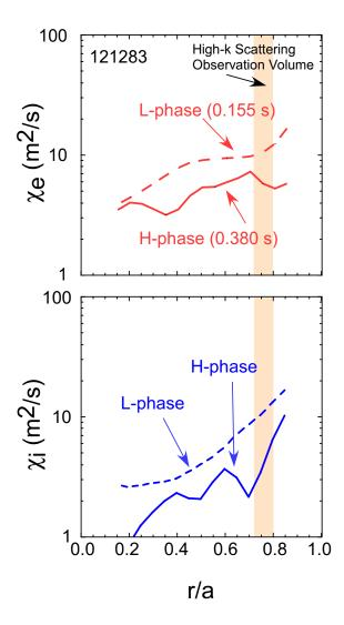
Figure 15: Electron (top panel) and ion (bottom panel) thermal diffusivities for the early L- (dashed curve) and H- (solid curve) phases of the discharge shown in Fig. 14. The ion thermal diffusivity is near the neoclassical level during the H-phase.
