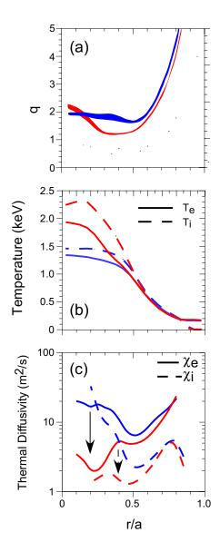
Figure 9: (a) q-profile comparisons for discharge with low central magnetic shear (blue) and strong reversed magnetic shear (red). (b) Electron (solid) and ion (dashed) temperature profiles for discharges shown in (a). (c) Electron (solid) and ion (dashed) thermal diffusivities for the discharges shown in (a).
