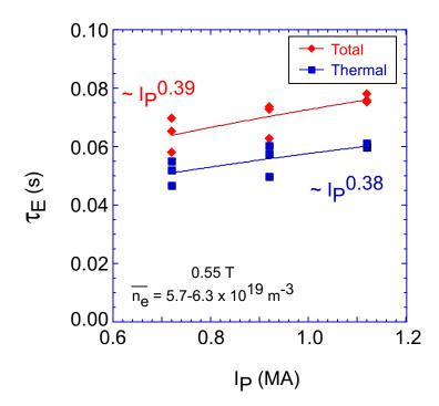
Figure 3: Total (red) and thermal (blue) energy confinement times vs  $I_p$  for the plasma current scan at constant toroidal field, density and heating power.
