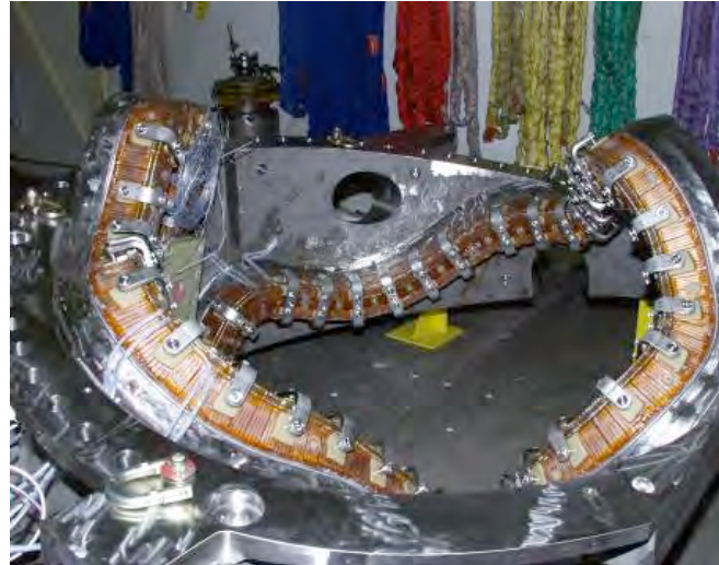
FIG. 4. Completed modular coil.
