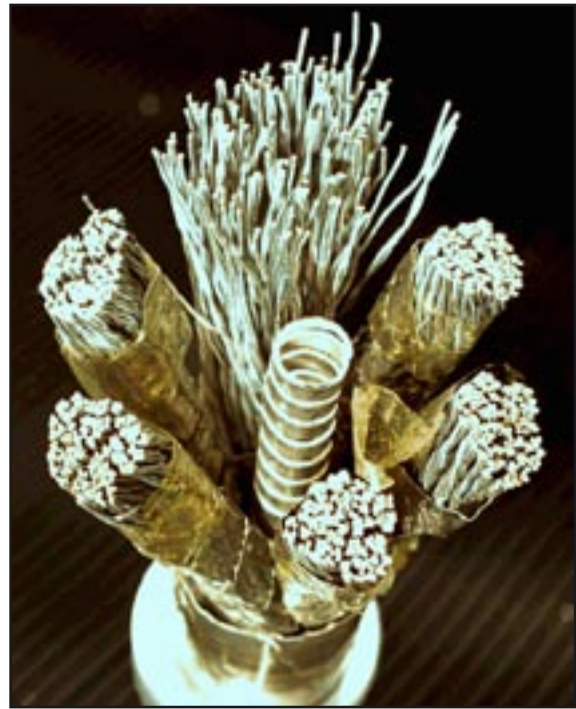
Figure 2. A sample end of the ITER toroidal-field conductor in conduit superconducting cables with one of the six bundles unbraided. The central perforated tube provides cryogenic cooling.
