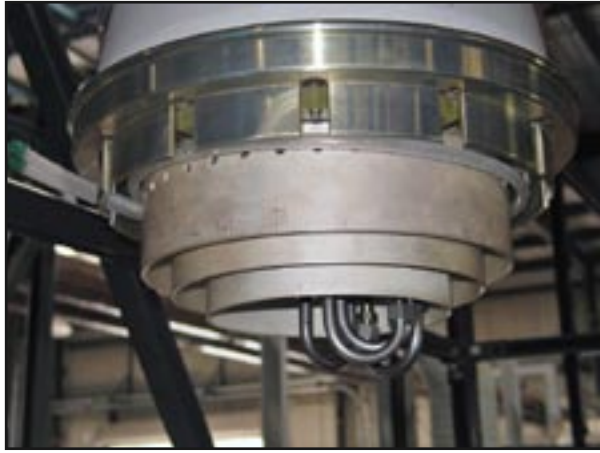
Figure 3. Completed socket assembly for the new radio-frequency high-power tube installation on DIII-D.
