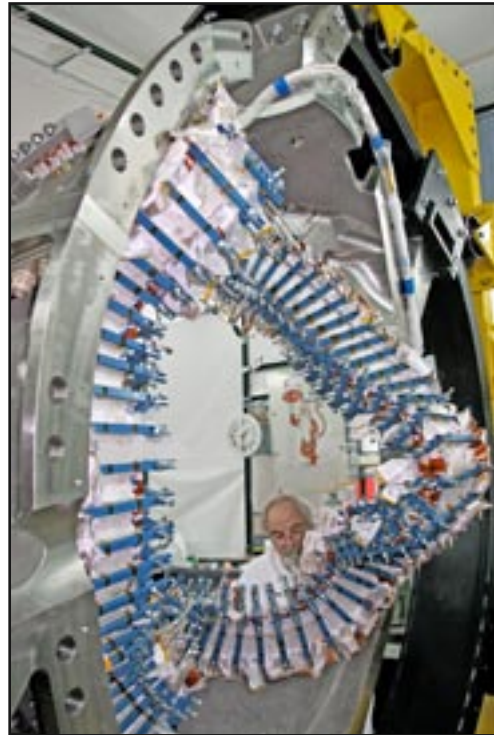
Figure 1. Fabrication of an NCSX modular coil.
