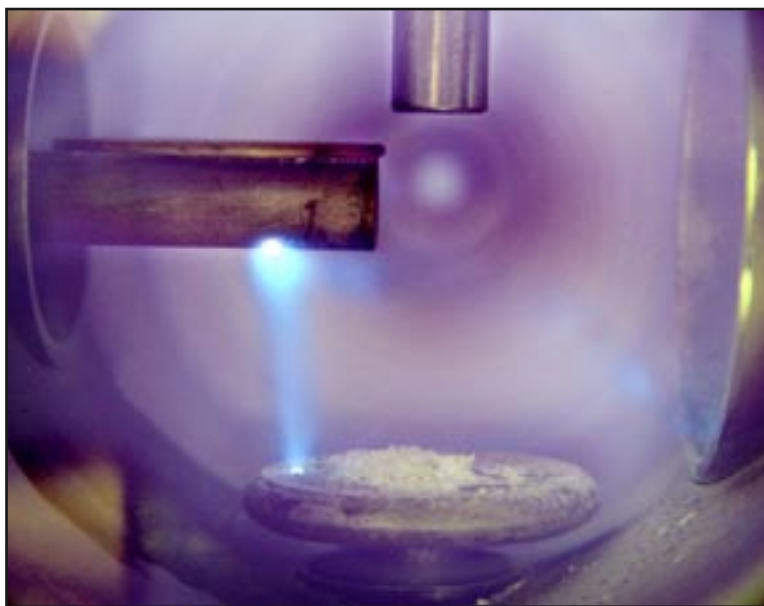
“Jump Start” from the 2006 Princeton University Art of Science competition by Elle Starkman and Andrew Zwicker. In the image, a pile of silica microspheres sits on a table and waits for the right combination of elements it needs to form a particle cloud suspended in plasma, which will float above the table as long as the plasma is maintained.
