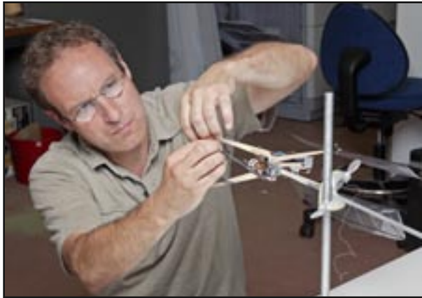
Figure 1. Dave Cylinder makes adjustments to the BITE mk 4. This version of a dual wing-pair air vehicle is being developed under PPPL's WFO Micro-aviation Vehicle project with the Naval Research Laboratory. Under this project fundamental research and development of the aerodynamics and airframes for unconventional miniature aircraft design are conducted.
