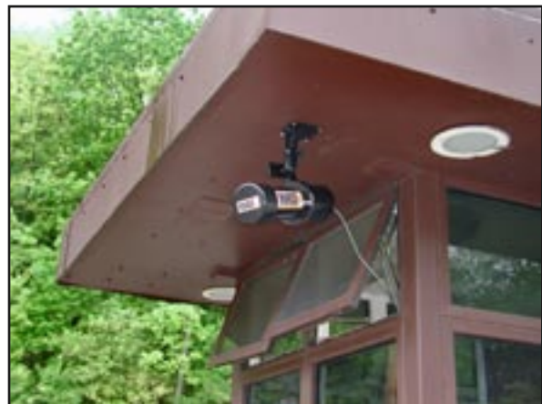
Figure 2. PPPL's Miniature Integrated Nuclear Detection System deployed at a guard station.
