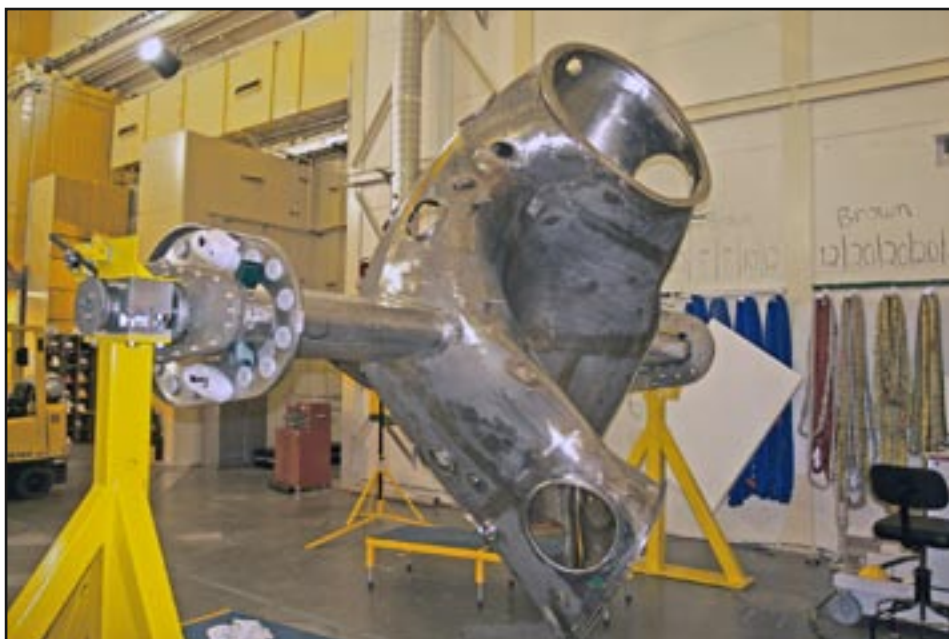
Figure 3. The NCSX vacuum vessel subassembly on a turning fixture.
