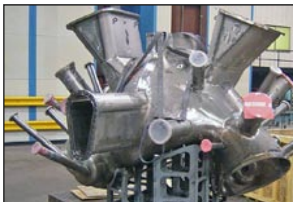
Figure 4. (top) Vacuum vessel design. (bottom) One of three field-period sectors with ports installed for vacuum testing.
