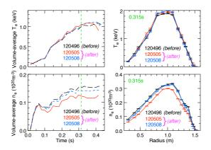
Fig. 6. Comparison of Thomson scattering profiles for NBI D reference discharges before (120496) and after (120505, 8) ohmic helium conditioning discharges applied to the graphite plasma facing surfaces. Pumping by the degassed graphite exhibited about an 18% decrease in density relative to the comparison discharge.
