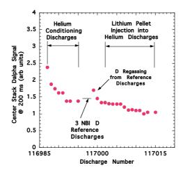
Fig. 1. Evolution of the representative level of  $D_{\alpha}$  luminosity from a sequence of 8 ohmic conditioning discharges (0.5 MA, 0.45 T), followed by 3 deuterium reference discharges, 4 additional ohmic clean-up discharges, and then 12 ohmic helium discharges, 9 of which with LPI of either 1.7, 3.4, or 5.0 mg. A small decrease in  $D_{\alpha}$  luminosity was evident in the discharges with LPI prior to the arrival of the LPI.
