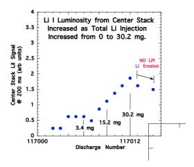
Fig. 2. The Li I luminosity from the center stack increased as the total lithium injection increased to 30 mg.
