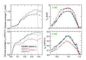
Fig. 5. Comparison of Thomson scattering profiles for NBI D reference discharges before (shot 120464) and after (120474, 5) lithium deposition following ohmic helium conditioning discharges. Pumping by the lithium coating on the conditioned graphite PFCs exhibited almost a 29% decrease in density relative to the comparison discharge
