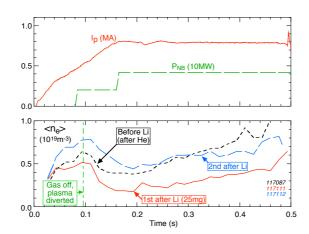
Fig. 4. Initial LSN NBI deuterium reference discharge (0.8 MA, 0.45 T) following 25 mg of lithium deposition on lower divertor exhibited a decrease in density by about 50%. Approximately 3.5 mg of  $D_2$  gas fueling is injected into each discharge.
