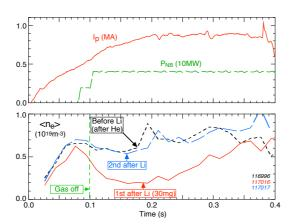
Fig. 3. Initial CSL NBI deuterium reference discharge (0.9 MA, 0.45 T) following 30 mg of lithium deposition exhibited a decrease in density of about 33% after termination of the initial gas puff. On the second discharge, the effect was less while on the third, the density was higher than before. Approximately 3.5 mg of  $D_2$  gas fueling was injected into each discharge.
