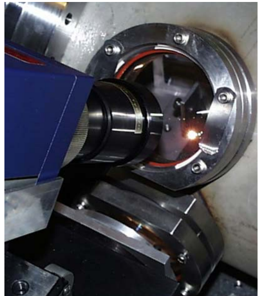
Fig. 3. Detritiation of TFTR Tile with Nd:Yag Laser
