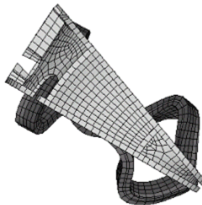
Fig. 6. For each shell segment, the modular coil protrudes outside of the shell edges.
