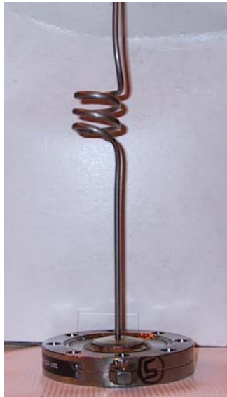
Fig.4. Photo showing the gas transport tube weld joint on the vacuum side of this flange and nearby strain relief coil.
