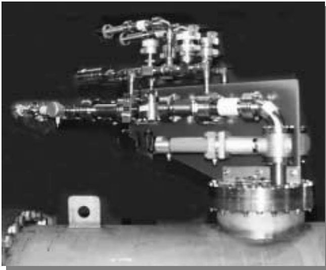
Fig. 2. The Bay L injector used for TMB injection during initial installation on the pumpduct. The gas injection assembly consists mainly of a piezoelectric pulse valve, interface valve, gas delivery line and pumpout line.
