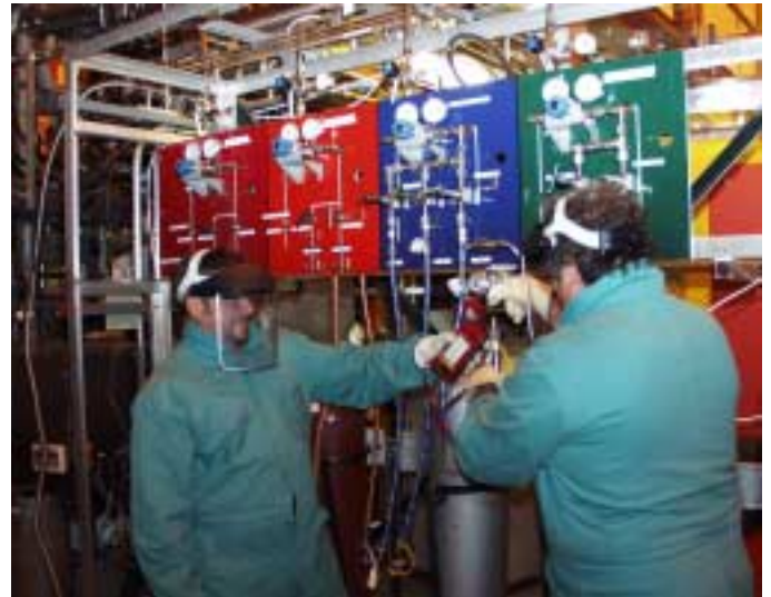
Fig. 3. Two TMB team members outfitted in the protective gear and with the gas sniffer for detecting any TMB during the process.
