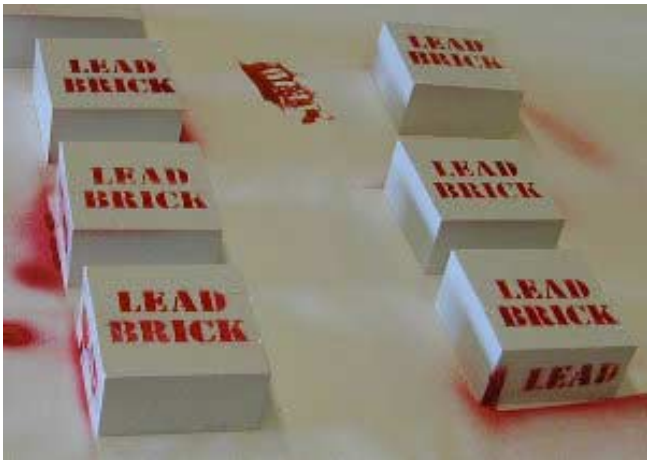
Fig.3 Lead bricks coated with polyurethane and labeled for future use.
