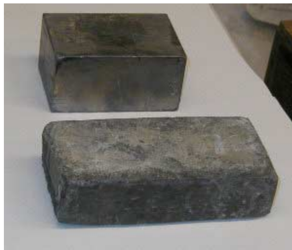
Fig. 1 the top lead brick exhibits no oxidized surface dust. The bottom lead brick exhibits oxidized surface dust.
