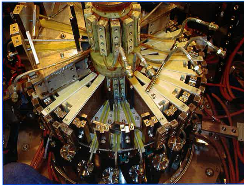
Figure 1. The partially disassembled National Spherical Torus Experiment hub assembly.
