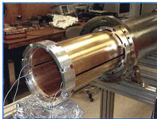
Figure 9. Electrode configuration in the Paul Trap Simulator Experiment.
