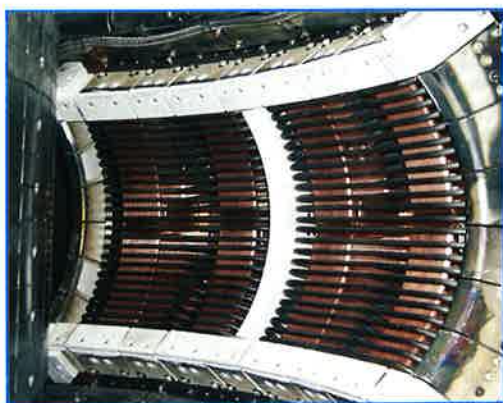
Figure 7. The 4-strap ion-cyclotron range of frequencies antenna with boron-nitride tiles and central septum.
