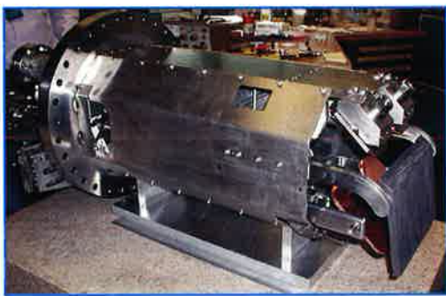
Figure 5. The second electron-cyclotron current-drive steerable launcher designed and built by PPPL for DIII-D.
