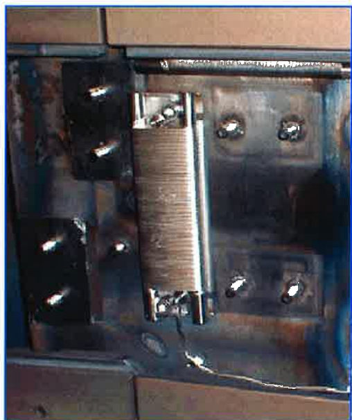
Figure 2. One of the poloidal magnetic field probes being installed in DIII-D.
