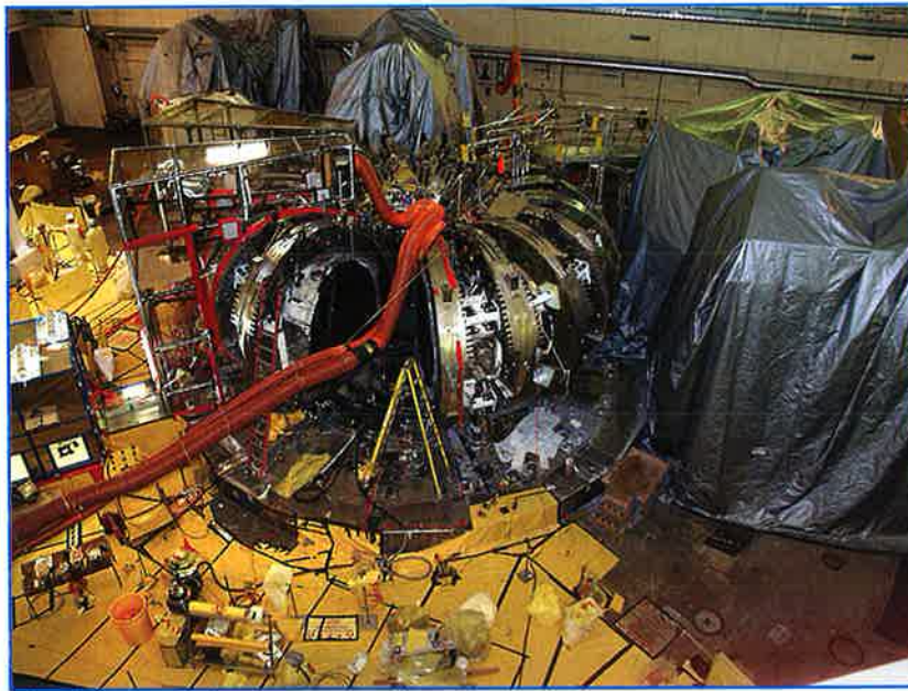
Figure 6. The Tokamak Fusion Test Reactor with the first sector removed.
