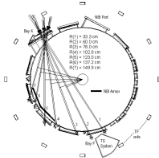
Fig. 1. Seven channel FIREtIP system will have fan view of beam lines. Three entrance windows and tangencies of each beam lines are provided
