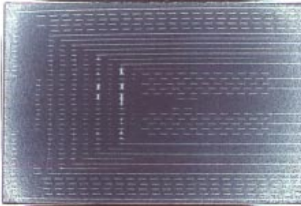
Fig. 7 Parts of a cross section (Y-Z plane) of an AT probe after co-firing. Horizontal 'lines' and 'dashes' are metallization seen in cross section. Thicker vertical 'lines' are vias seen in cross section.
