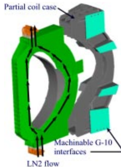
FIG. 3. TF COIL AND CASE DETAILS
