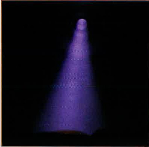
Figure 6. View (looking into nozzle) of an argon plasma expanding from the nozzle.
