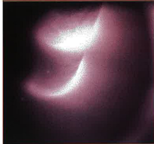
Figure 5. Image of the liquid lithium limiter taken through a lithium filter. The view shows the surface that faces the plasma at a framing rate of 1,000 frames per second. The emission is most conspicuous at the plasma contact point (upper band) and the tip of the limiter heat (lower band).
