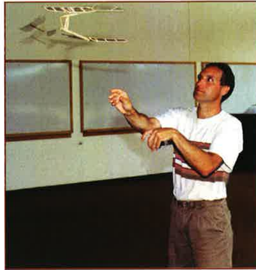
Figure 3. PPPL researcher David Cylinder is creating innovative bird-like airframes for micro aircraft vehicles, which would carry sensors for intelligence gathering and radar jamming. He is shown here with his Samara model which looks like two winged seeds that counter rotate. The name comes from the samara seed — such as that of a maple tree — which has a wing like a single-bladed rotor.
