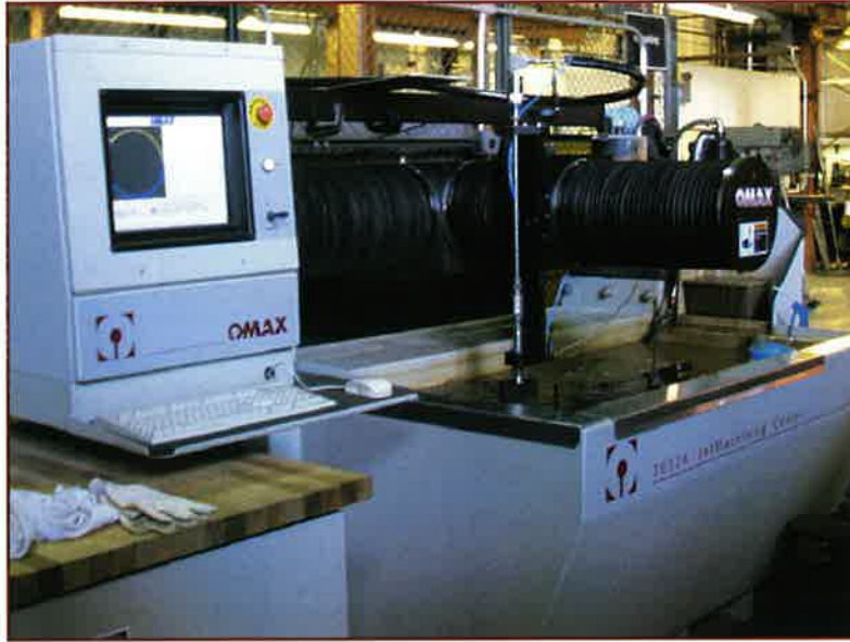
Figure 5. PPPL's new water-jet machining center.
