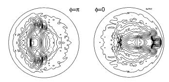
FIG. 1. Pressure contours during a high- $\beta$  disruption for a reversed shear plasma. Nonlinear development of a ballooning mode produces pressure steepening in the normal shear region with a structure which looks like fingers in 2D and ribbons in 3D. This can cause magnetic field line stochasticity and a thermal quench.
