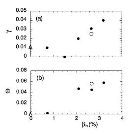
FIG. 4. (a) Growth rates, and (b) rotation frequencies of m=1 internal modes at various  $\beta_h$  values of the fusion alphas, obtained from MHD (triangles), from the gyrokinetic-energetic-particle/MHD hybrid model (solid circles), and from the gyrokinetic-particle-ion/fluid-electron hybrid model (open circles).
