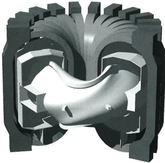
Figure 1. Machine concept for 1999 NCSX reference design using PBX-M toroidal field coils. Shown installed are the three-dimensional vacuum vessel, three-dimensional coil support shell, and cryostat.
