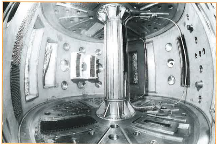
Figure 2. Interior of CDX-U vacuum vessel, showing rotatable antenna with insulating shield (light color).
